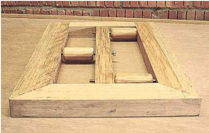
▲ Pic.6 The plinth is a simple construction, but the wheels make the bureau easier to move
